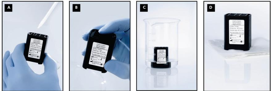
**Cleaning procedure for PyroMark Q24 Cartridge.**
