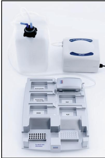
The mains plug should be easily accessible in case the vacuum pump needs to be disconnected quickly from the mains power.
