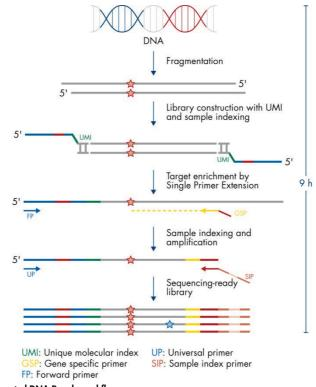
Figure 2. QIAseq Targeted DNA Panels workflow.
