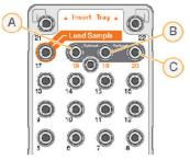
A Position 18 for Read 1 Custom Primer Figure 10. MiSeq reagent cartridge. A: Position 18 for Read 1 Custom Primer; B and C: not relevant.
