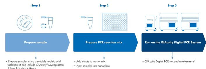
QIAGEN's mycoplasma detection workflow in three steps. Step 1: Nucleic acid extraction with spike-in of Internal Control during the lysis step. Step 2: Setup of dPCR reaction with up to 22.6  $\mu$ L sample and transfer to a 26k Nanoplate. Step 3: One-step reverse transcription dPCR run on the QIAcuity instrument and subsequent data analysis using the QIAcuity Software Suite.
