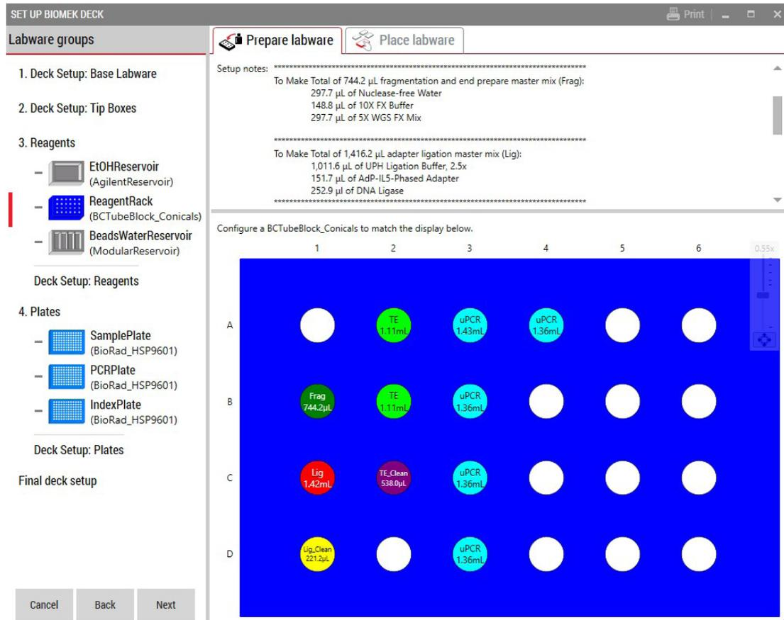
Figure 5. Guided Labware Setup displays reagent volumes and guides the user for correct deck setup.
