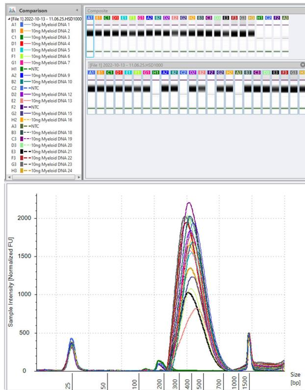
**Figure 6.** Library yield analyzed on TapeStation 4200 with High Sensitivity D1000 screening tape. Traces are overlaid with non-template controls (NTC).
