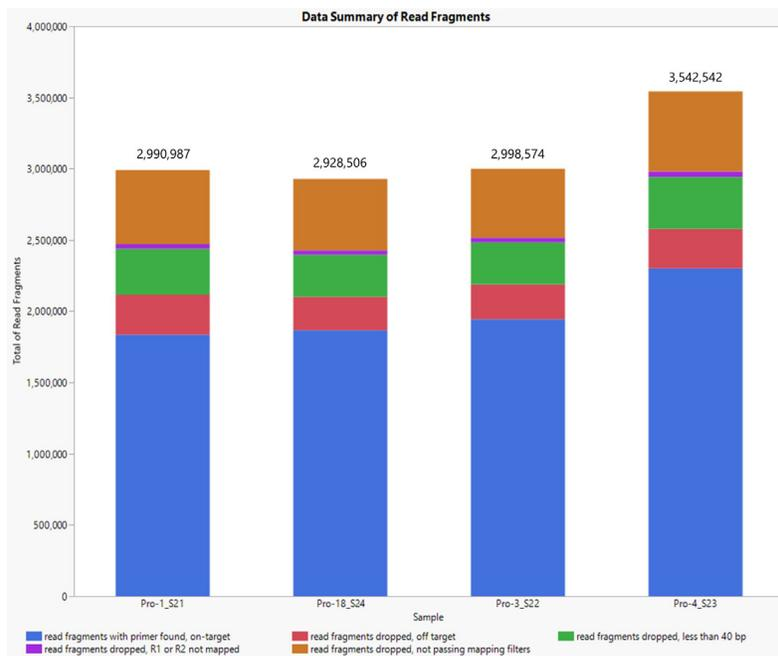
**Figure 7.** Alignment statistics for each of the QIAseq® Targeted DNA Pro libraries sequenced. The total number of reads is displayed above the stacked bar for each sample. This graph shows the classification breakdown for all fragment reads. The total number of read fragments exceeded 2.9M and the percentage aligned to the targeted sequence attributed to over 86% of the total read fragment count.
