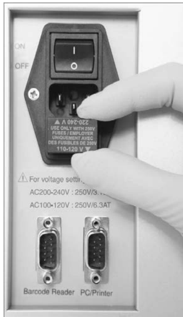
Selecting the correct fuse for 100–120 V line power supply.
