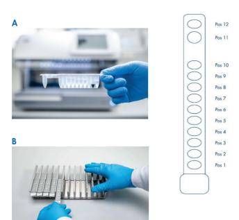
Figure 1. Ease of worktable setup using reagent cartridges. A: A sealed, prefilled reagent cartridge (example). B: Loading reagent cartridges into the cartridge rack. The cartridge rack itself is labeled with an arrow to indicate the direction in which reagent cartridges must be loaded.
