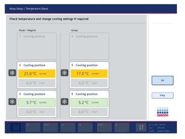
The QIAsymphony AS automatically starts cooling the loaded cooling positions. The current temperature of the cooling positions is updated in real time. If the current temperature is outside the target temperature, the slot will appear yellow. If the current temperature is within the target temperature the slot will appear green.
