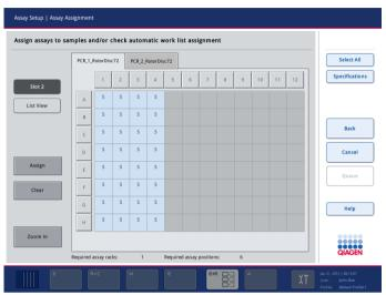
Assay Assignment screen with no work list assigned and Yes selected for Assign each assay individually?
