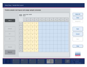
**Note**: To delete sample position(s) that have been assigned, select the position(s) and press **Clear**.
