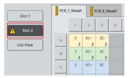
**Note**: If there is insufficient space in the assay racks or reagent holder, or if insufficient adapters have been configured to process the defined samples, the corresponding drawer button will flash yellow. Pressing this button will display hints about what to do.
