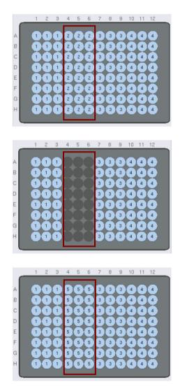
Be aware that, if the original SP batch only covered 2 columns and not 3 columns (e.g., if the original SP batch contained 9 samples), the maximum number of samples that can be reloaded equals the number of positions in the 2 free columns (i.e., 16). If an attempt is made to reload more than 16 samples, the following error message will appear:
