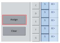
The selected Assay Parameter Set(s) will be assigned to the selected positions. A number will appear in the bottom right corner of the assigned sample positions. This number indicates the number of Assay Parameter Sets that have been assigned to a particular sample.
