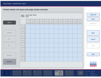
Sample Rack Layout screen, with no rack file assigned.
