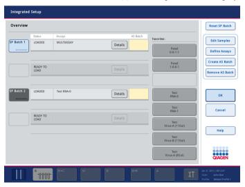
Press Create AS Batch. An AS batch will be created from the selected SP batches. A number will appear in the AS Batch column. This number indicates which AS batch a particular SP batch is linked to.
