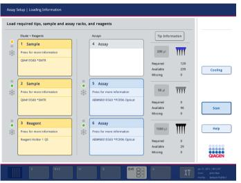
Loading Information screen with assay racks assigned to slots 5 and 6.
