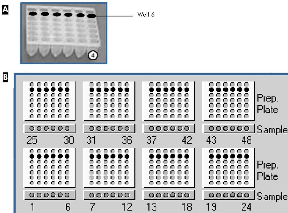
**Figure 1. Adding internal control to sample preparation plate.** **A** Sample preparation plate. **B** Worktable overview for 48 processed samples. Black dots indicate positions where diluted internal control should be added.
