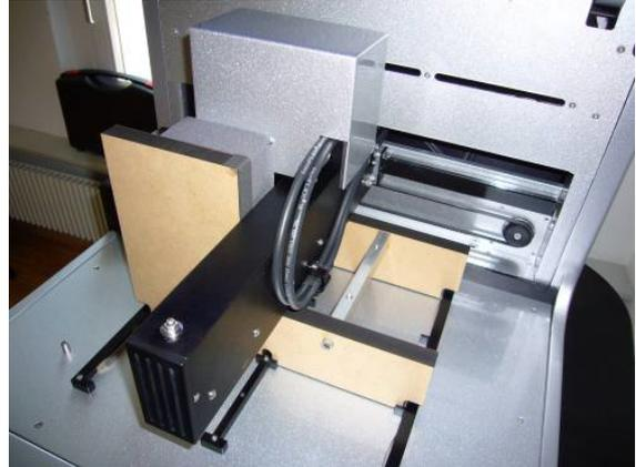
2. Move the pipettor head to the right and remove the transport lock from the worktable.
