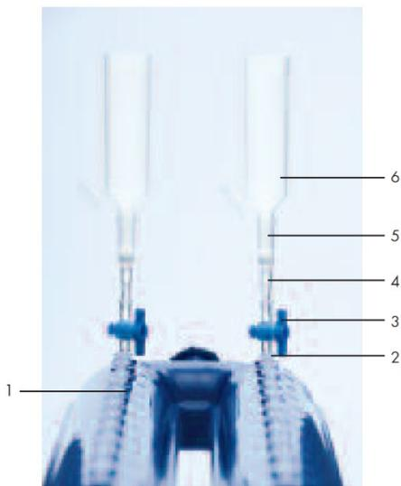
**Figure 4. Setting up the QIAvac 24 Plus with QIAamp Mini columns using VacValves, VacConnectors, and Tube Extenders.**
