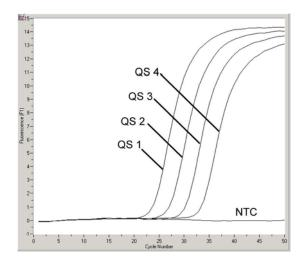
Fig. 7: Detection of the Quantitation Standards (WNV LC/TM QS 1 – 4) in fluorimeter channel F1. NTC: no template control (negative control).
