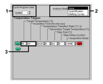
Fig. 4: Initial Activation of the Hot Start Enzyme.
