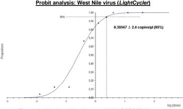
Fig. 9: Analytical sensitivity of the artus WNV LC RT-PCR Kit.
