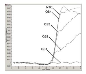
Fig. 8: Detection of the Internal Control (IC) in fluorimeter channel F3/Back-F1 with simultaneous amplification of Quantitation Standards (WNV LC/TM QS 1 – 4). NTC: no template control (negative control).
