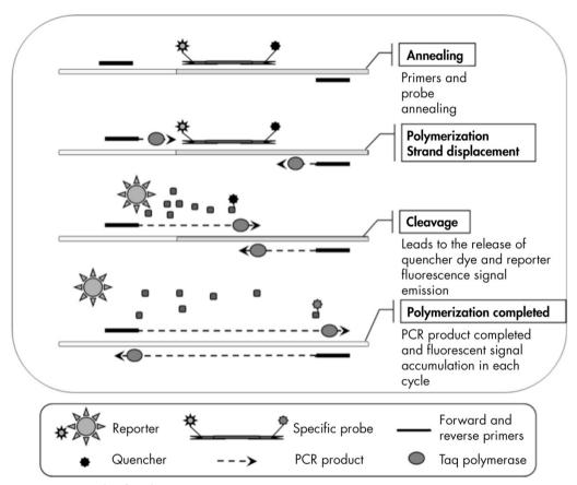
Figure 1. Principle of real-time PCR reactions.
