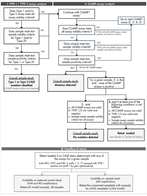
Figure 6. Decision flowchart to determine CALR mutation status of test samples.
