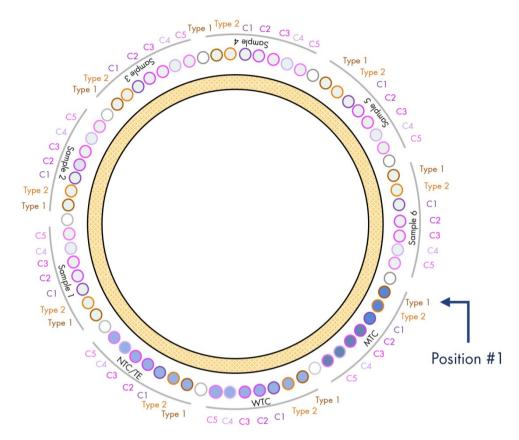
Figure 5. Suggested rotor setup for an experiment with the CALR RGQ PCR Kit.
