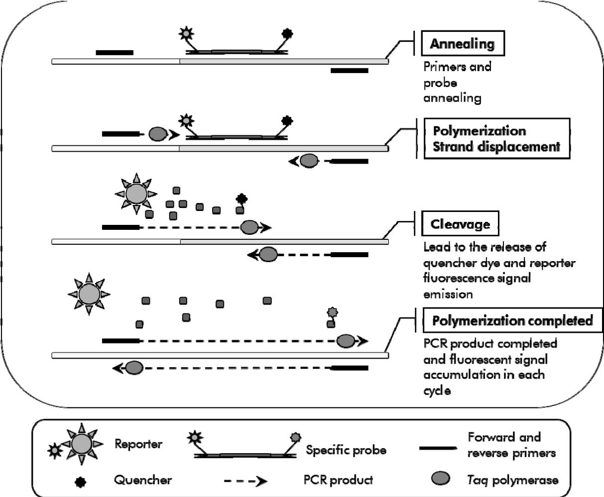
Figure 1. Reaction principle.
