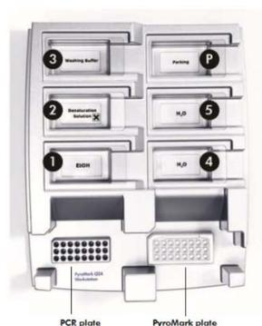
**Figure 23. Positions on the PyroMark Q24 Vacuum Workstation.**
