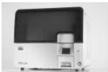
Figure 1. The QIAcube. Circulating nucleic acid purification using the QIAamp Circulating Nucleic Acid Kit can be partially automated on the QIAcube.
