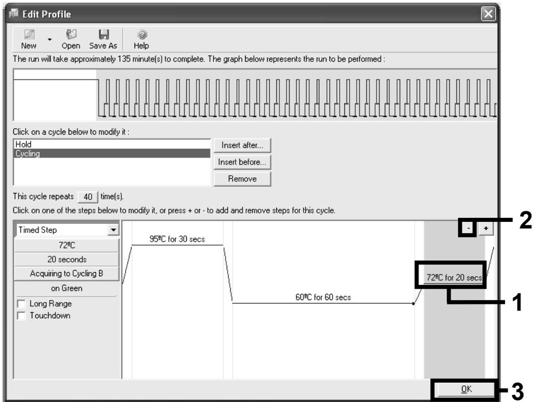
Figure 9. Removal of extension step.
