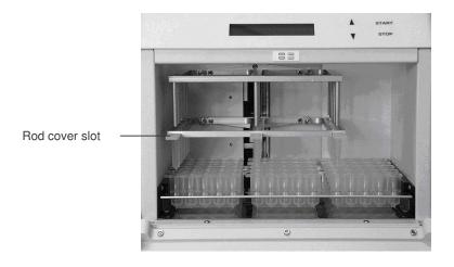
Insert a 5-rod cover into a rod cover slot so that the short tab faces inward and the long tab faces outward. 5-rod covers must be inserted so that they click into place.
