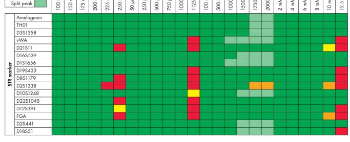
Overview of the Investigator ESSplex Plus inhibitor resistance. The assay was tested with 4 inhibitors (humic acid, hematin, tannic acid, and indigo carmine). 500 pg of Control DNA XY5 was used as template and PCR was performed under standard conditions. 100 RFU was used as the threshold for allele calling.
