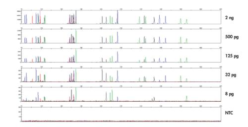
Sensitivity study of the Investigator ESSplex Plus Kit. Different concentrations of Control DNA XY5 were used as a template. Samples were amplified on an ABI GeneAmp PCR System 9700 Thermal Cycler with gold-plated silver block. Analysis was performed on an AB Genetic Analyzer 3500, equipped with a 36 cm 8-capillary array and POP-4<sup>™</sup> polymer. NTC: No-template control (pelase add to end of last sentence
