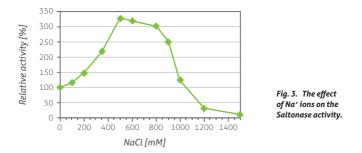
Saltonase is active in a broad range of Na $^{+}$  ions' concentration with optimum activity between 0–1100 mM (over 80% of Standard Activity) and maximum activity at 500 mM of NaCl.
