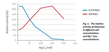
Saltonase's activity graph, depending on NaCl and  $Mg^{2*}$  ions concentration in the buffer, determines optimum reaction conditions.
