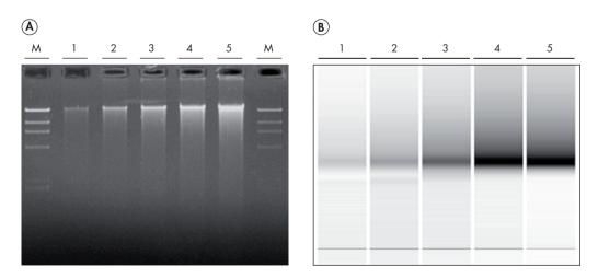
Figure 1. Electrophoresis of samples from a dilution series. A Lanes 1–5: gDNA samples at respective concentrations of 10, 25, 50, 75, and 100 ng/μl run on a 1% agarose gel for 150 min at 80 V. Lane M: lambda HindIII size marker. B The same samples run using a QIAxcel DNA Screening Cartridge and the AM900 method.
