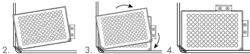
Examples of acceptable microplate loading configurations:
