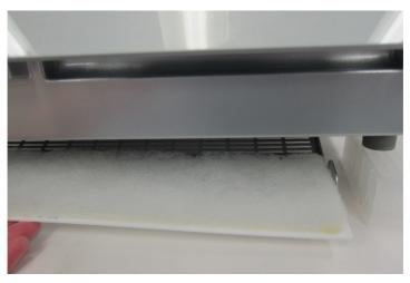
4. Replace with a new filter and push the compartment to the top to close.
