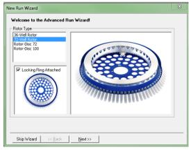
Select the correct rotor and confirm the locking ring is attached.
