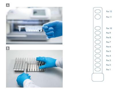
Figure 1. Ease of worktable setup using reagent cartridges. (A) A sealed, prefilled reagent cartridge. Fill levels vary, depending on the type of reagent cartridge. (B) Loading reagent cartridges into the cartridge rack. The cartridge rack itself is labeled with an arrow to indicate the direction in which reagent cartridges must be loaded.
