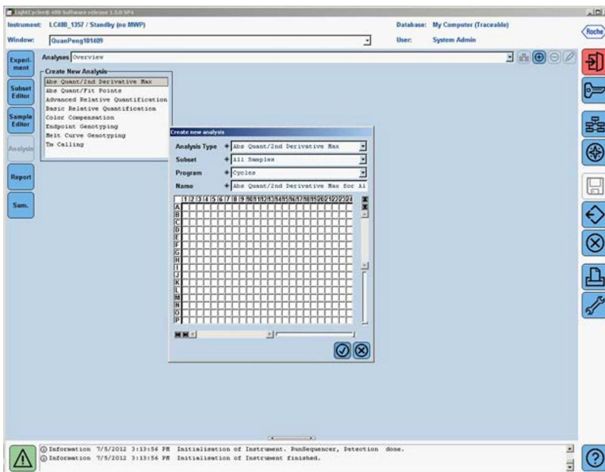
Figure 9. Setting up the analysis for the second derivative maximum.
