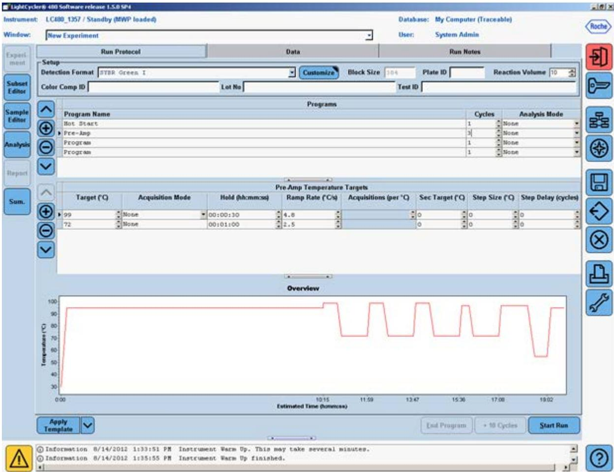
Figure 4. Setup of the second program — “Pre-amp Cycling.”
