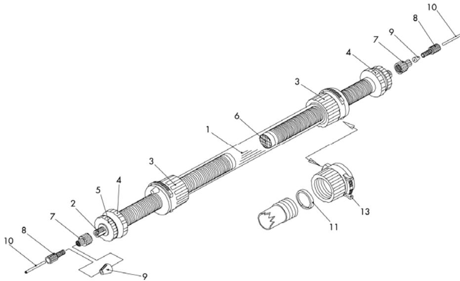
**Components of the Vantage L Laboratory Column VL 44 x 25, (cat. no. 96440250).**
