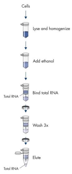
Figure 1. QIAwave RNA Mini procedure.
