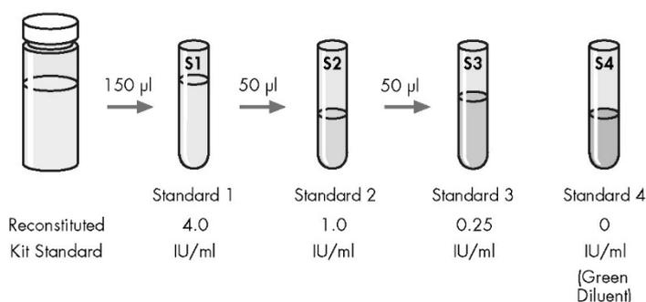
Figure 2. Preparation of standard curve.
