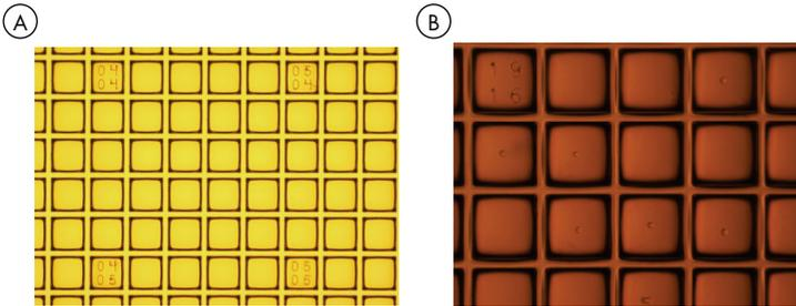
**Figure 1.** A. Numbered microwells on the QIAscout array. B. Microwells containing single cells.
