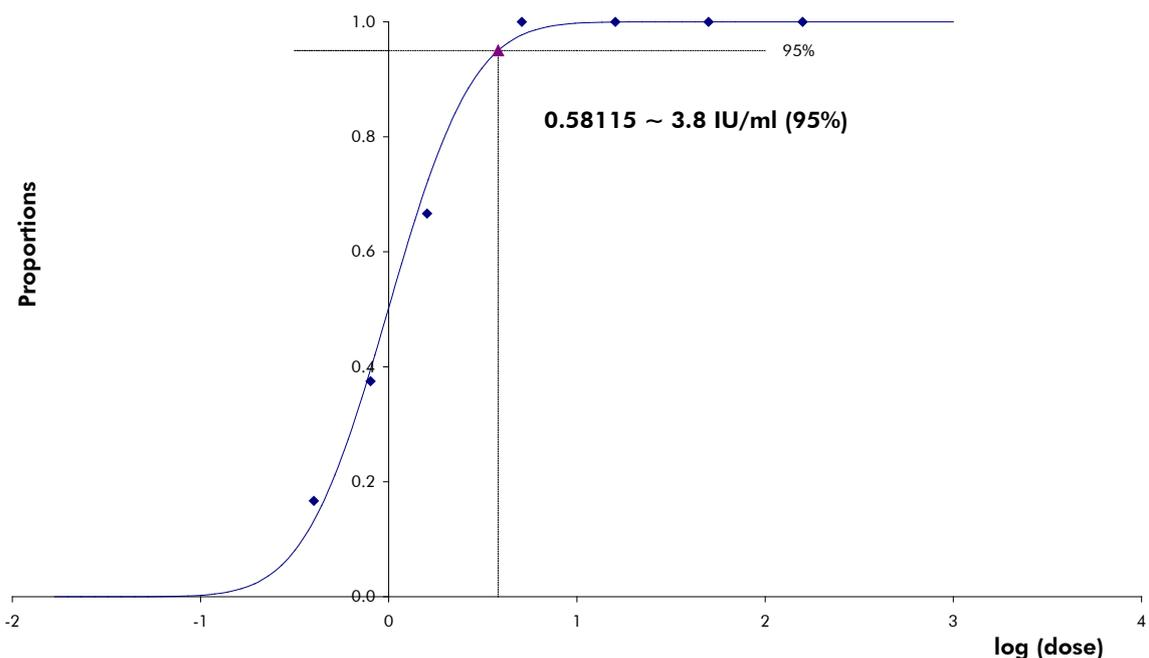
**Figure 1. Probit analysis: HBV (Rotor-Gene 3000).** Analytical sensitivity in consideration of the purification (QIAamp DSP Virus Kit, QIAGEN) of the *artus* HBV RG PCR Kit on the Rotor-Gene 3000.
