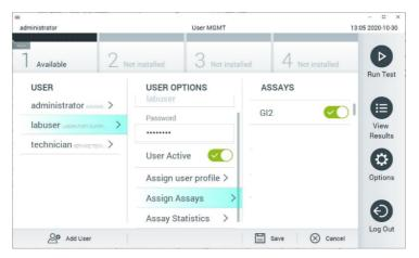
Figure 58. Assigning the active assay.
