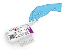
Figure 4. Opening the sample lid of main port.
