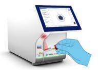
Figure 10. Scanning sample ID bar code.
