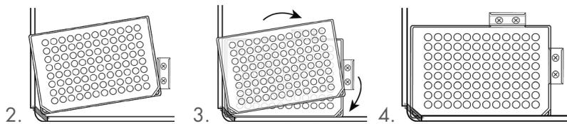
Examples of acceptable microplate loading configurations:
