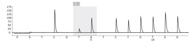
Figure 10. Pyrogram trace obtained after analysis of samples with a GTG  $\rightarrow$  GAG mutation in base 2 of codon 600 (nucleotide 1799).
