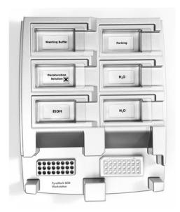
Figure 3. Placement of PCR plate and PyroMark Q24 plate on the vacuum workstation.
