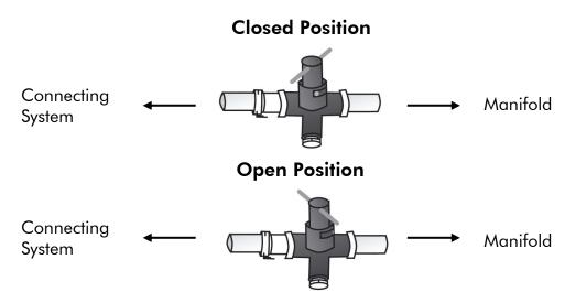
**Figure 6** Main vacuum valve in the closed and open position.
