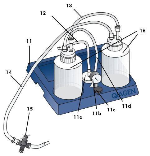
Figure 4C Setting up the QIAvac Connecting System.
