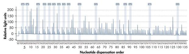
Analysis of 16 CpG sites in a long sequence run. The PyroMark<sup>®</sup> Q24 Advanced increases both read length and reliability of methylation analysis at positions later in the sequence. This example demonstrates 135 nucleotide dispensations and the accurate analysis of 16 different CpG positions in a single PyroMark Q24 Advanced CpG reaction. The PyroMark instrument delivers highly reproducible real-time quantification of methylation frequencies at individual CpG sites.
