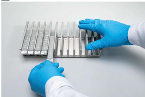
Figure 2. Ease of worktable setup using reagent cartridges. (A) A sealed, prefilled reagent cartridge. Fill levels vary, depending on the type of reagent cartridge. (B) Loading reagent cartridges into the cartridge rack. The cartridge rack itself is labeled with an arrow to indicate the direction in which reagent cartridges must be loaded. Each reagent cartridge contains 12 individual positions.
