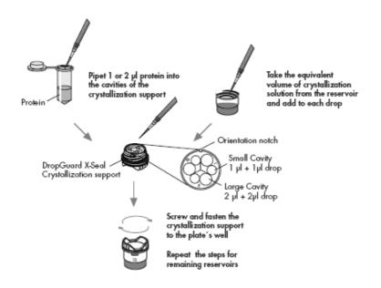
Figure 2. Setting up crystallization trials using DropGuard crystallization supports.
