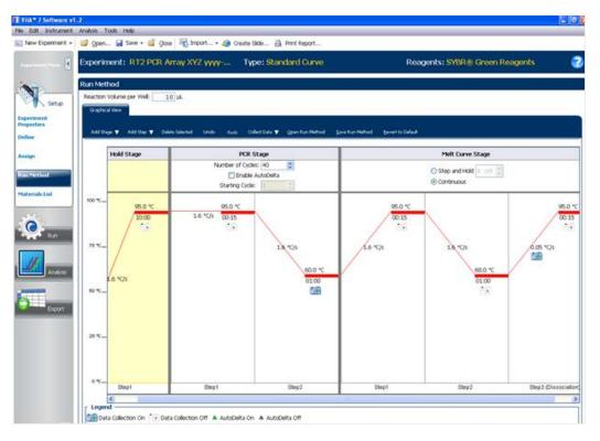
Figure 4. "Run Method" tab.
