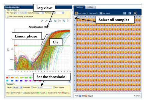
Figure 7. Setting the threshold.
