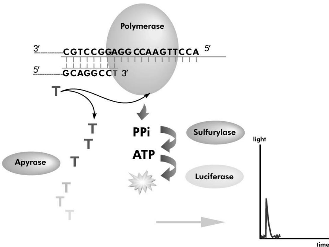
**Figure 1. Schematic illustration of the Pyrosequencing cascade.** As nucleotides are incorporated into the analyzed DNA strand, pyrophosphate is released and converted to ATP. Generated ATP drives the light reaction detected as a peak on the Pyrogram. Apyrase degrades any unincorporated nucleotides.
