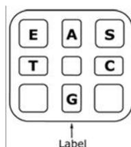
**Figure 2. Illustration of the PyroMark Q24 Cartridge as seen from above.** The annotations correspond to the label on the reagent vials. Add enzyme mixture (E), substrate mixture (S), and nucleotides (A, T, C, G).
