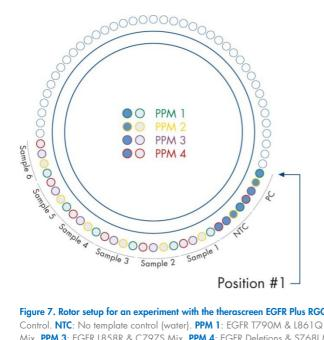
Figure 7. Rotor setup for an experiment with the therascreen EGFR Plus RGQ PCR Kit. From position 1 PC: EGFR Positive Control. NTC: No template control (water). PPM 1: EGFR T790M & L861Q Mix. PPM 2: EGFR Insertions & G719X Mix. PPM 3: EGFR L858R & C797S Mix. PPM 4: EGFR Deletions & S768I Mix. Sample 1 to Sample 6: DNA samples. Note: All remaining positions O should be filled with empty tubes.
