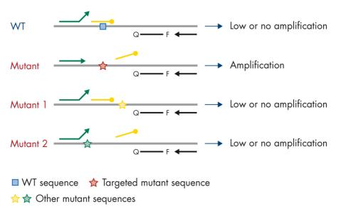
Figure 4. Mutation detection by clamp technology. WT: Wild type. Q–F: Double-dye probe. D: Forward and reverse primers.
