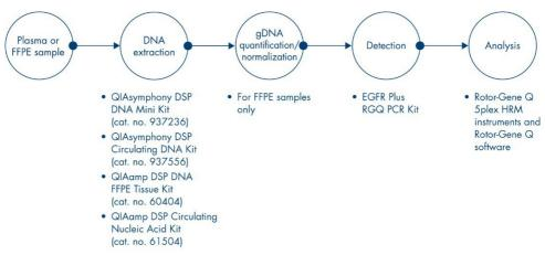
Figure 1. EGFR Plus RGQ PCR Kit workflow. For non-DSP extraction kits, see "Materials Required but Not Provided", page 21.
