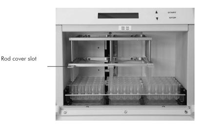
Insert a 5-rod cover into a rod cover slot so that the short tab faces inward and the long tab faces outward. 5-rod covers must be inserted so that they click into place.
