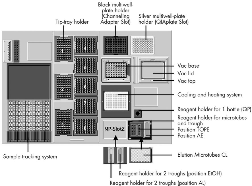
Figure 1. Overview of the BioRobot MDx worktable.
