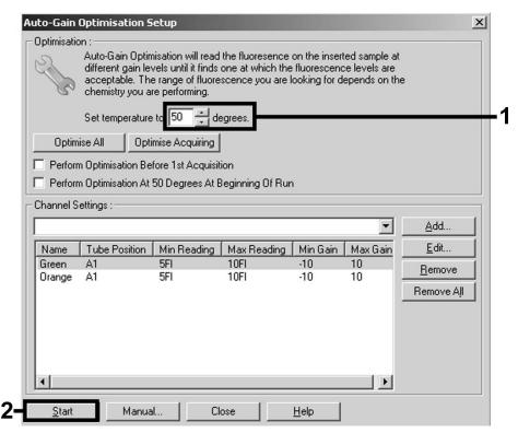
**Figure 7. Adjusting the fluorescence channel sensitivity.** Screenshot for the *artus* HI Virus-1 QS-RGQ Kit is shown as an example. **Note**: This step may differ for other *artus* QS-RGQ Kits. See Table 2 for the specific information for each *artus* QS-RGQ Kit.
