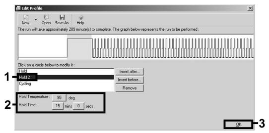
**Figure 5. Initial activation of the hot-start enzyme.** Screenshot for the *artus* HI Virus-1 QS-RGQ Kit is shown as an example. **Note**: This step may differ for other *artus* QS-RGQ Kits. See Table 1 for the specific information for each *artus* QS-RGQ Kit.
