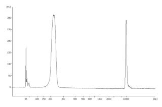
Figure 1. Agilent trace data showing the correct size distribution of library fragments and the absence of adapters or adapter-dimers.
