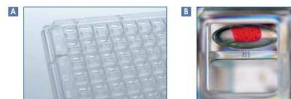
**Features of the NeXtal Evolution Phase  $\mu$ plate.** These include a groove for easy cutting of tape, a broad rim to avoid evaporation, and a unique "half American football" shaped protein well. **A** The NeXtal CubicPhase  $\mu$ plate. **B** Top view of the oval-shaped well coated with MO. For better visualization, the MO has been colored with a red dye.
