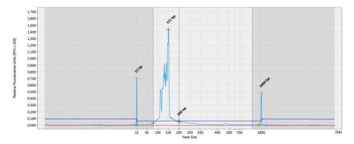
Figure 4. Trace data from the QIAxcel Advanced capillary electrophoresis instrument, showing the pooled and purified multiplex PCR product of the GeneRead QIAact Actionable Insights Tumor Panel (GRTP-101X). A peak observed at approximately 150 bp represents the amplicons.
