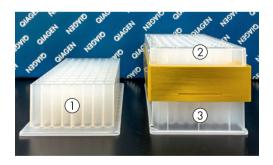
Figure 7. Filtered lysates were collected in a 2 ml plate, then filtered cells were transferred to a Plasmid *Plus* 96 Plate on top of a drip tray using an adapter. 1: Filtered lysate with Buffer BB added. 2: Plasmid *Plus* 96 Plate. 3: Drip tray.
