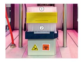
Figure 6. Both plates were then placed onto the Resolvex A200 to clarify the lysates using positive pressure. 1: TurboFilter 96 Plate. 2: S-Block.
