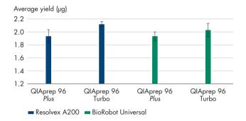
Figure 11. Comparison of yields and CVs across a 96-well plate for plasmid DNA extracted using different protocols on the Resolvex A200 and the BioRobot Universal workstations.
