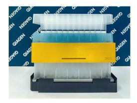
Figure 3. TurboFilter 96 Plate placed on top of a QIAprep 96 Plate and deep-well plate with adapters.
