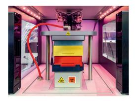
Figure 4. QIAprep 96 Plate placed for DNA binding and washing steps, using adapters to fit under the pressure head.
