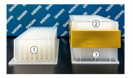
Figure 5. Lysis and neutralization were performed in 2 ml plates, then lysed cells were transferred to a TurboFilter 96 Plate located on top of a collection plate with an adapter. 1: Buffer S3 added to lysed cells (Buffer P1 and P2 added earlier). 2: TurboFilter 96 Plate. 3: S-Block.
