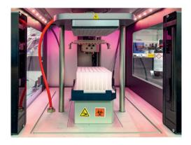
Figure 2. Buffer dispensing to resuspend, lyse and neutralize cells using Resolvex A200 (shaking performed offline).
