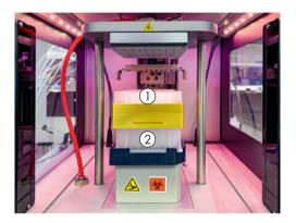
Figure 8. Both plates were then placed onto the Resolvex A200 to load samples onto the sorbent via positive pressure. 1: Plasmid *Plus* 96 Plate. 2: Drip tray for discarding flow-through.
