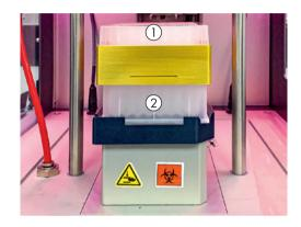
Figure 9. Plasmid Plus 96 Plate and elution plates were placed on the Resolvex A200 for dispensing of Buffer EB. A slow pressure gradient was applied to elute the samples. To maximize recovery, the elution step was performed twice. 1: Plasmid Plus 96 Plate. 2: Elution plate.
