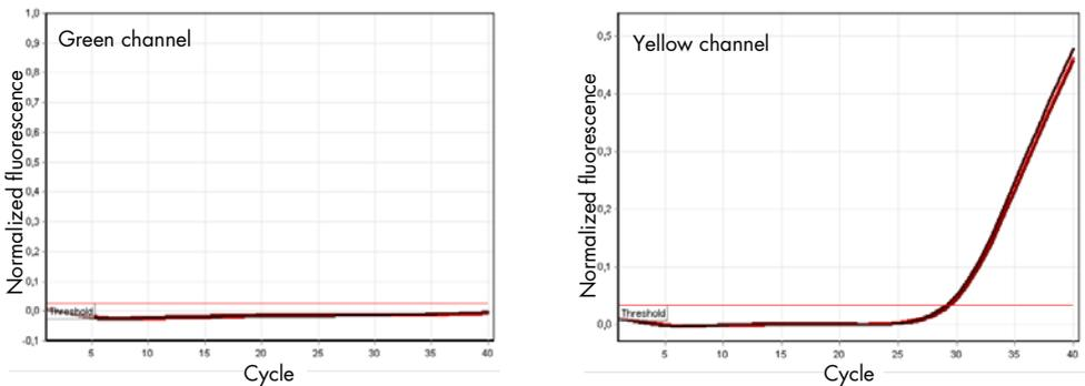
**Figure 1. The sample is negative for the tested GMO or genetic construct.** The 3 sample curves in the green channel (left) are at the baseline and below a preset threshold. The corresponding curves of the internal control in the yellow channel (right) are above the threshold, indicating that the PCR was successful.
