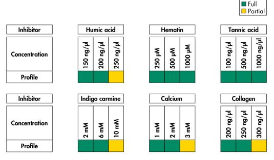
Figure 4. Investigator ESSplex Plus inhibitor resistance. The assay performance was tested in the presence of increasing concentrations of 6 types of inhibitor. 500 pg of Control DNA 9948 was added to the master mix and PCR was performed under standard conditions. The analysis was performed on an Applied Biosystems 3500 Genetic Analyzer using the Investigator IDproof Software. 100 rfu was used as the threshold for allele calling.
