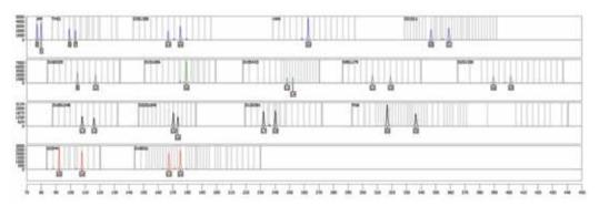
**Figure 3. Investigator ESSplex Plus inhibitor resistance.** The electropherogram displays a profile of 500 pg Control DNA XY5 generated in the presence of 500 μM Hematin. The analysis was performed on an Applied Biosystems 3500 Genetic Analyzer using the Investigator IDproof Software.
