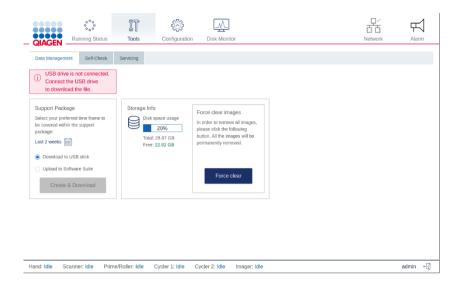
3. To clear the data, tap **Force clear images**. Click **OK** in the confirmation dialog box to delete the data. Images from the system and database will be removed.
