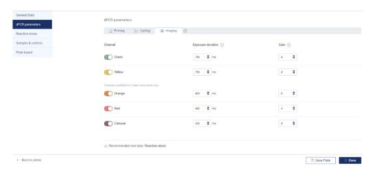
The Imaging tab enables you to set the respective exposure duration and gain value for each channel. The channel options depend on the connected instrument. QIAGEN offers QIAcuity One in 2-plex and 5-plex version. QIAcuity Four and QIAcuity Eight offer 5-plex analysis. The following table shows the available channels provided in each instrument.
