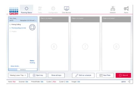
To view more details about the run, tap **Show details**. The dialog box appears containing information about the plate (in the General Data tab), as well as each step of the run (in the dPCR Parameter tab).
