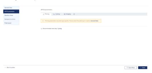
You can set up the run profile of your experiment in the dPCR parameters tab. This tab is divided into three subtabs: Priming, Cycling, and Imaging.
