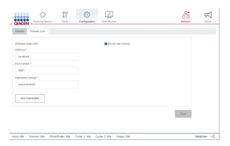
5. Enter the IP address in the address field of the Software Suite URL section.
