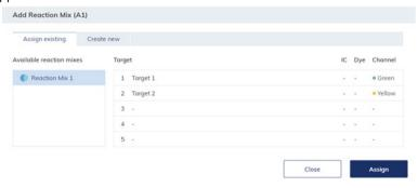
Select the reaction mix you want to add to the plate. To create a new reaction mix, click the Create new tab. See Defining reaction mixes for information about creating a new reaction mix.
