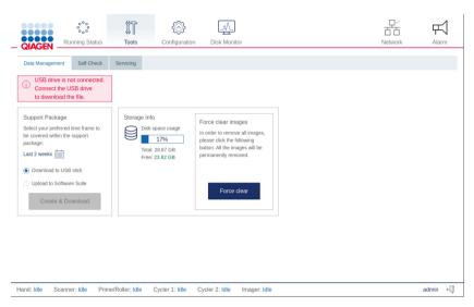
Connect a USB drive to the instrument. Wait for the device to detect the USB drive. A notification is displayed once the drive is connected.
