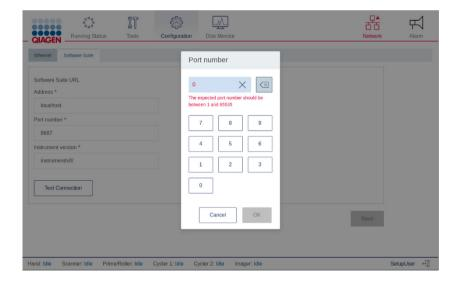
**Note**: To get the IP address of the Suite Server, the instrument must be connected to the Suite Server. From your Home screen, click the Windows icon and navigate to **Command Prompt**, or enter **cmd** in the Search field. A command line window appears. Enter **ipconfig** to view the network settings.
