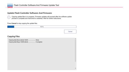
**Note**: If an error occurs when the files are being copied, an error message is shown on the screen. Tap **Cancel** to stop the process. Remove the USB drive and tap **Reboot** to restart the instrument. If the QIAcuity does not function after an unsuccessful software update, contact QIAGEN Technical Services.
