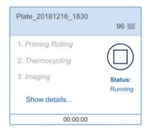
Aborting a plate during the priming/rolling step renders it unusable and the plate cannot be used and run again. A plate that has been aborted during the Thermocycling or Imaging step can be used again. To rerun the plate, configure a run with only the remaining steps. See section Rerunning a plate for more information.
