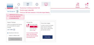
In case of 2 and 3, additional information is shown to inform about the actions that should be taken to gain the disk space: forcing the clearing of images, which haven't been transferred to Software Suite or setting up a connection with Software Suite.
