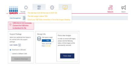
3. Red - when the remaining free disk space is less than 4 GB (~14%)
