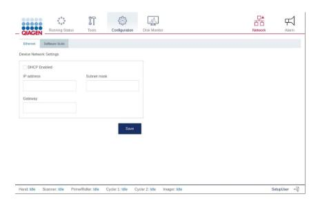
4. Check the **DHCP Enabled** box. If you check this box, the IP address and MAC address fields are disabled. The assigned IP and MAC addresses of device are displayed in the **IP address** and **MAC address** fields.
