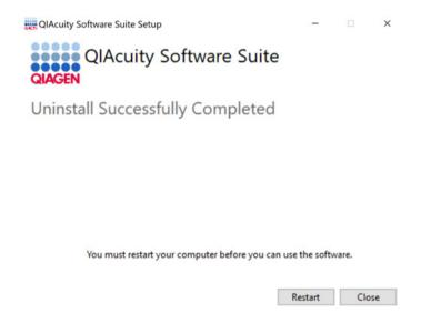
**Note**: After uninstalling the Software Suite, the User database remains on the computer prevailed. In order to remove it, go to **C:\ProgramData\Qiagen** and remove the **\Qiaidentity** directory manually. Be aware that **\ProgramData** might be hidden and you need to change the view settings of the explorer. Please also manually delete the remaining PostgreSQL, which is located at **C:\Program Files\PostgresSQL**.
