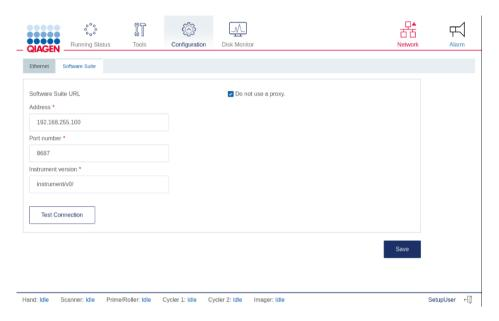
**Note**: An error message displays if the address and port number you entered are invalid. Tap **OK** to close the error message, and then re-enter the correct address and port number in the address field in the **Software Suite URL** area.
