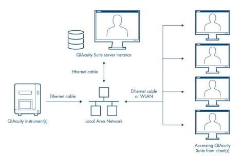
The QIAcuity instrument(s) and QIAcuity Software Suite are installed to a network, allowing multiple clients to access the QIAcuity instrument(s) via a single QIAcuity Suite server.
