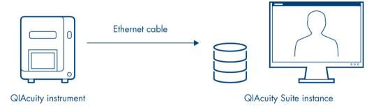
The QIAcuity instrument and QIAcuity Software Suite are connected via Ethernet cable.
