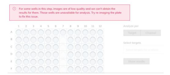
In case more than one imaging step has been done, the imaging step where the low signal quality occurred is marked in red and the message is shown when moving the mouse over the camera icon.
