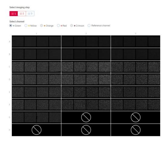
**Note**: Errors affecting single wells or empty wells are indicated by a symbol in the affected well. Try reimaging the plate with different exposure and/or gain settings. If the error persists, create a support package and contact QIAGEN Technical Services.
