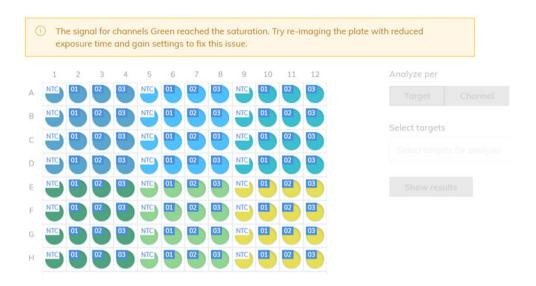
In case more than one imaging step has been done, the imaging step where the saturation occurred is marked in yellow and the warning message is shown when moving the mouse over the camera icon.
