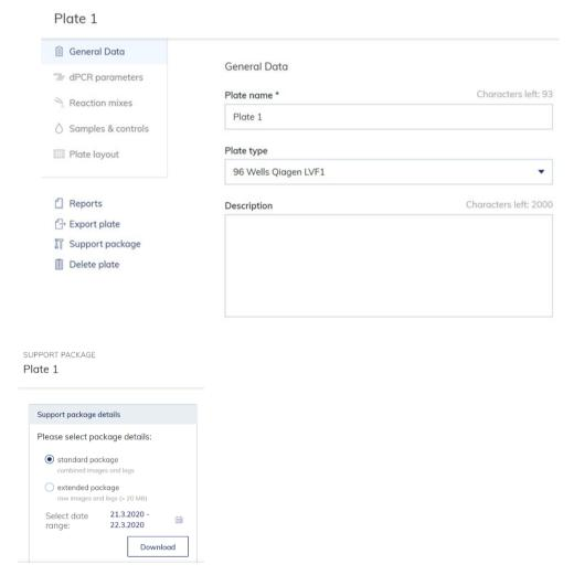
**Note**: The standard package includes the log files and a combined image view of all wells. The extended package includes the log files and the raw images of each single well. By clicking on the calendar symbol, you can define the time frame from which the support package shall be generated. Click **Download** to download the support package as zip file.
