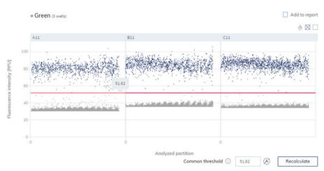
The 1D Scatterplot view with Common threshold.
